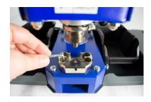
9. Loosen the two front screws on the lower bracket.
