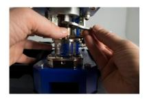
2. Actuate the manual operating lever to drive the finger guard downwards.
