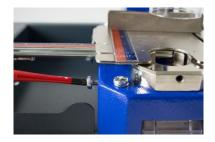
4. Fix the spacer with the left screw.
