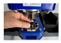
7. Insert the lower die into the hole and press up to the stop.
