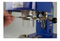
2. Make certain that the adapter nut is firmly tightened, using the open-end spanner supplied.
