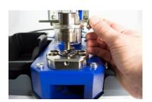
14. Drive the finger guard with the manual operation lever slowly downwards and control that the upper die is centred in the lower die without snagging. If this is not the case, adjust the die as described in Section 5.1.
