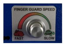
The speed with which the finger guard moves down can be adjusted with the setting screw. This can compensate for differences in the compressed air supply. Rotating in the clockwise direction reduces the speed. This adjustment affects only the use of the footpedal.
