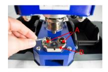
4. If necessary, loosen the two Allen screws A and slide the lower bracket B together with the die to the correct position.
