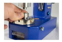
7. Insert the lower die into the hole and press up to the stop.
