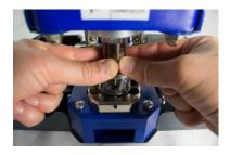
10. Pull the upper die downwards with the fingers and move the lower bracket so that the upper die fits into the hole of the lower die without snagging.
