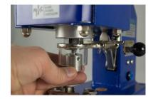
3. Drive the finger guard upwards and turn out the upper die completely.
