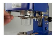
5. Actuate the manual operating lever to drive the finger guard downwards.
