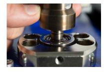
3. Check the position of the upper die relative to the lower die. The dies must be exactly centred over each other and the upper die must fit into the lower die without snagging.
