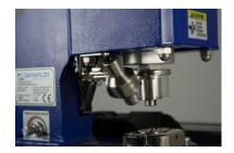
3. Attach the Laser pointer on the screw, but don't yet tighten the nut.
