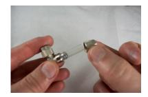
4. Cut away a piece (approx. 25mm long) of the compressed air hose (not supplied) and attach it to the angular piece supplied.
