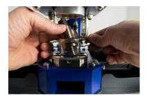
3. Actuate the manual operating lever to drive the finger guard downwards.
