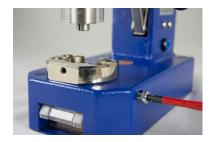
5. Loosen the right screw for the lower die with a screwdriver.
