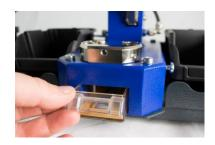
4. Remove the punch waste collecting container. Press the lower die upwards with the finger and remove the die.
