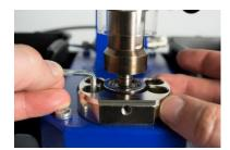
5. Tighten the two front screws on the lower bracket.
