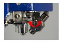
6. To adjust towards the left and right rotate the pointer. The Phillips-head screw is the fulcrum and under the wing screw is an elongated hole for adjusting the position.
