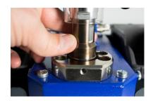
6. Slide the upper die several times completely into the lower die and control that the upper die is centred in the lower die without snagging.
