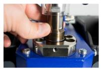
12. Slide the upper die several times completely into the lower die and control that the upper die is centred in the lower die without snagging.
