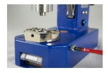
8. Tighten the screw for the lower die and then check the adjustment as described in Section 5.1. Faulty adjustment causes poor results and can damage the die.
