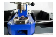
8. Tighten the screw for the lower die.
