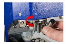
5. To adjust towards the front and rear rotate the bracket in the horizontal plane.
