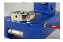
4. Loosen the right screw for the lower die with a screwdriver.
