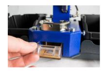
5. Remove the punch waste collecting container. Press the lower die upwards with the finger and remove the die.
