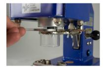
2. Remove the adapter nut using the open-end spanner.
