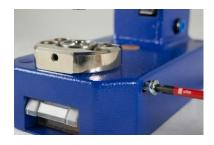
3. Loosen the right screw for the lower die with a screwdriver.
