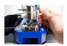
8. Slowly drive the finger guard downwards with the manual operating lever and control that the upper die is centred in the lower die without snagging. If this is not the case, adjust the die as described in Section 5.1.
