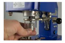
3. Actuate the manual operating lever to drive the finger guard upwards and turn out the die completely.
