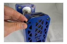
2. Remove the four plastic feet on the lower side.
